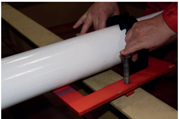
Once the pipe has been lifted, the rubber element can be removed
