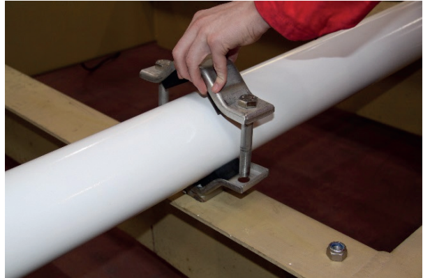
Remove the bolts, and lift of the upper steel body part. The lower part is welded to the structure.
