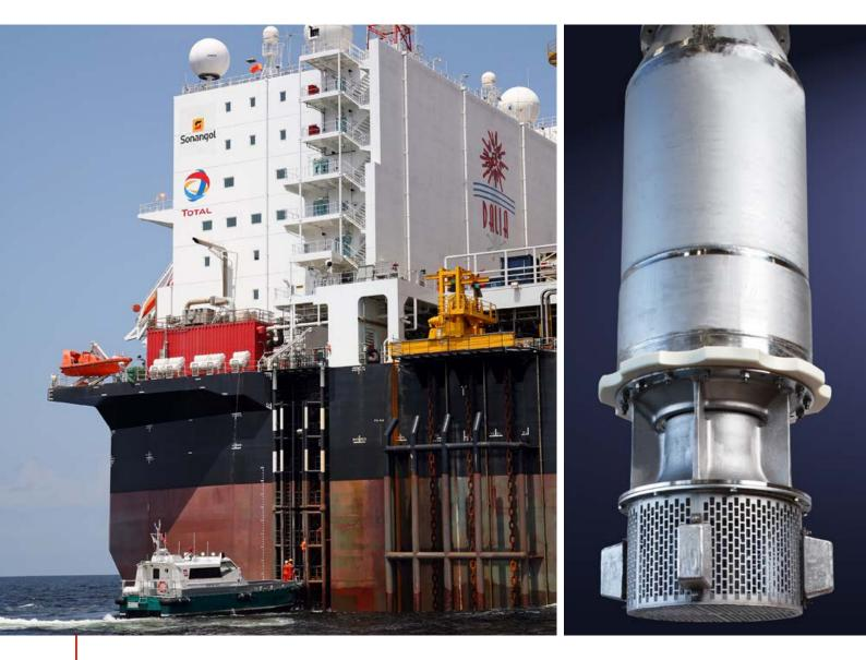
Rapid response pumping systems for firefighting Framo diesel-hydraulic fire water pumps
