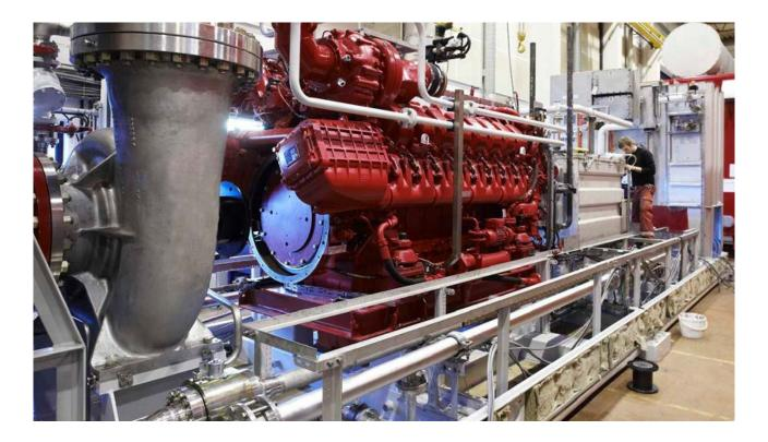
The diesel engine is fitted with auxiliary equipment to comply with the requirements of NFPA 20, main classification societies and national authorities.
